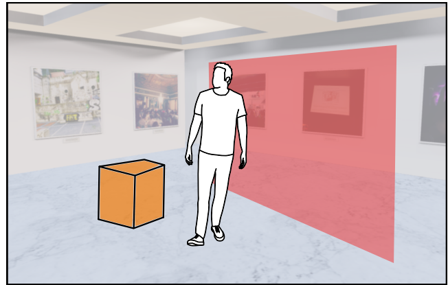
Figure 1: To achieve safe walking in VR, our approach combines Walking-In-Place locomotion technique with Natural Walking and virtual proximity indicators for obstacles and room boundaries.
